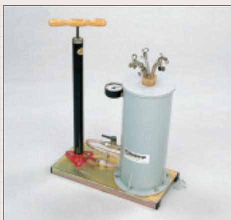
Vacuum tank with vacuum pump
