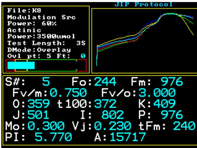
*The OS-30p+ actually measures  $F_O$  using a weak modulated red light. It is not an estimated value.*
