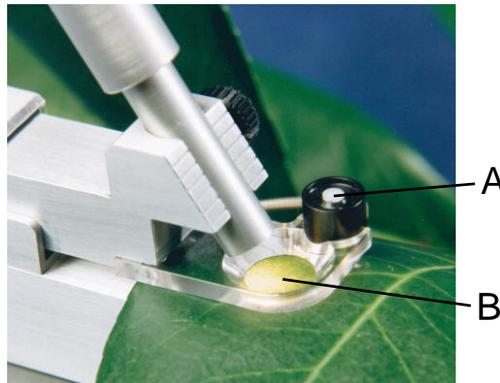
**Fig. 1-7B.** *The PAR sensor (A) located in the cup on the lower section of the clip. This position is suitable for actinic light calibration (described below) or simultaneous PAR monitoring during analysis of narrow samples (B) which do not cover the sensor in this position.*
