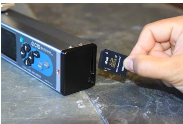
Figure 5. SDcard and USB cable connection for CI-203
