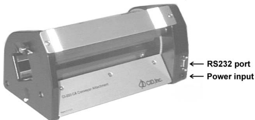
Figure 9. The RS232 port and the Power Jack of the CI-203CA.
