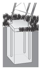
The B18's stakes embed in a concrete pad.
