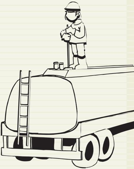
When the tank bottom sampler touches the bottom it is filled with the liquid from the bottom.
